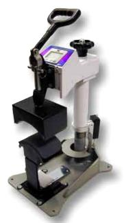
Make sure the lower pedestal is adjusted and slid forward or backward to line up with the heat platen above.
