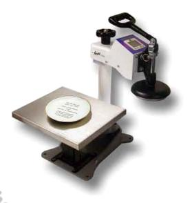
Plate the black circular silicone pad on the tray. Center the pad so that it is directly underneath the plate heater block attachment when swung over. Make sure it lines up directly under the plate heat platen. Then peel the backing off the circular black silicone pad and permanently stick it to the tray.
