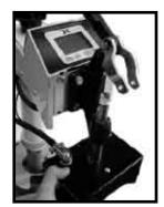
Reattach the quick release pin through the linkage and the heat platen shaft.
