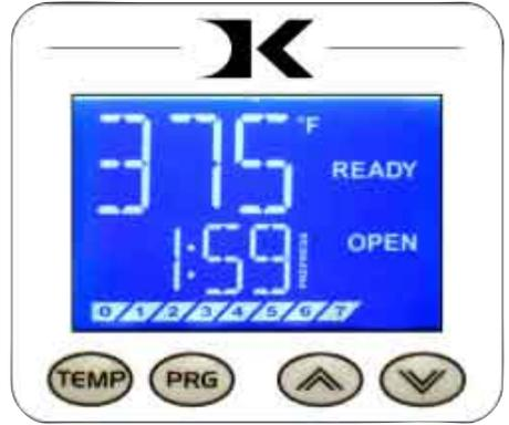
The right side the screen will indicate the heating status by stating HEATING, READY, both of those words, or none at all,
