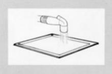
Spray the screen with water. It should be completely wet, but not dripping. Place screen on Yudu lid, with the backside facing up.
