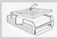
Apply generous bead of ink onto screen just above design. Make sure bead of ink is at least as wide as design.
