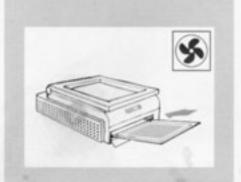
Place screen in drying rack of Yudu machine. Press fan button and let the screen dry for 15-20 minutes. Machine will beep when done. Test for dryness before moving on to the next steps.
