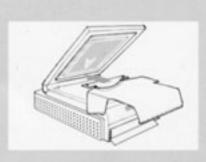
Tape the front of the screen around edges to seal any open screen areas.
