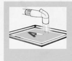
Spray screen with cool water to remove green emulsion from design area. It may be necessary to gently rub both sides of screen by hand or use a sponge to remove emulsion in detailed design areas.
